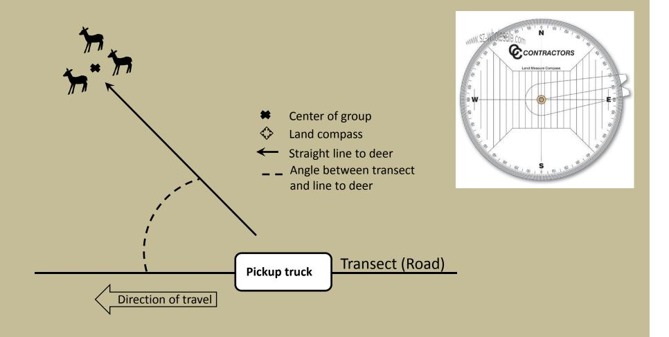
Calculation of the azimuth using a land compass for distancebased sampling techniques used during deer survey
